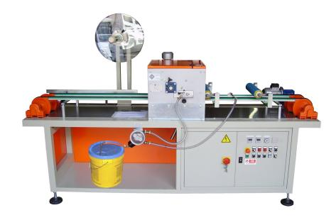
The automatic machine mod. SG2005S glues the mosaic onto kraft paper and fibreglass netting. The main adjustments can be made on the **control panel**, such as the length and position of paper and fibre, plus the amount of glue on the dispensing roller can be adjusted without having to stop production as what happens in many cases.
